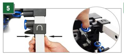
While putting the Extended Leg Attachments into the frame, squeeze the two black buttons at the tip to allow entry into the frame. Pull the pull pin ring on the frame so the Extended Leg Attachment will go in smoothly.
