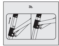
and one hand on the leg and pushing up until the slider "clicks" in place.
